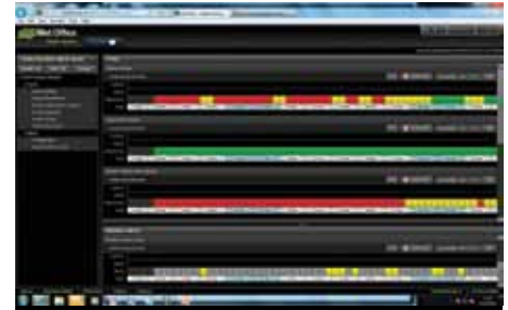
▲ The Met Office Weather Windows tool uses a traffic-light system to identify the optimum time for defined site tasks over the next 14 days
